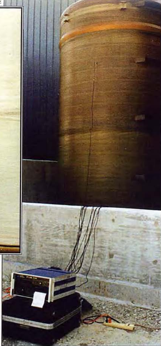
FIGURE 1 (above). AE testing doesn't require much set-up beyond attaching piezoelectric sensors to the shell of the tank
