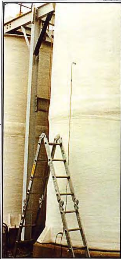
FIGURE 1 (above). AE testing doesn't require much set-up beyond attaching piezoelectric sensors to the shell of the tank
